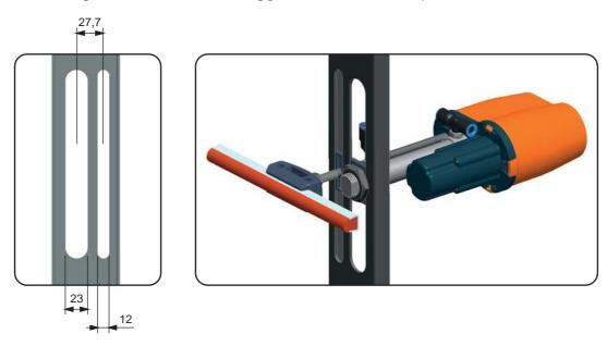
Example of installation of  $\mathbf{SGA}^{\mathsf{TM}}$  system (  $\mathbf{Side}\ \mathbf{Guide}\ \mathbf{Adjustment}^{\mathsf{TM}}$  ) on an air conveyor.
